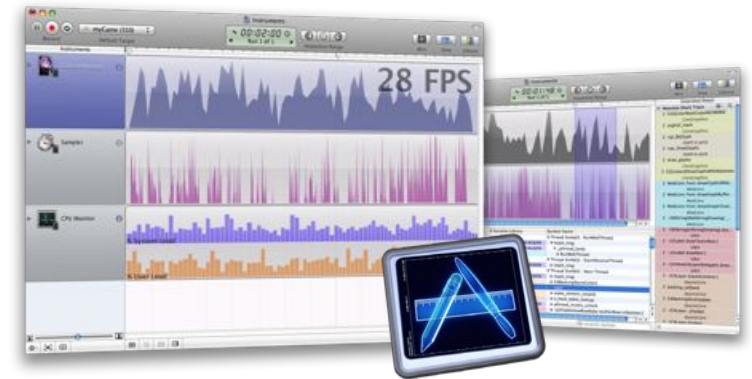
Instruments collects and displays data in real time, such as disk, memory, or CPU usage, making it easy to pinpoint problem areas.
